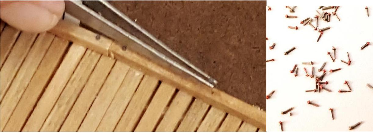
Drill a .025 hole with pin vise and drop in the NBW with tweezers. They are hardly visible on top of the 6" x 6" Safety Bollard. Rust and weather.
